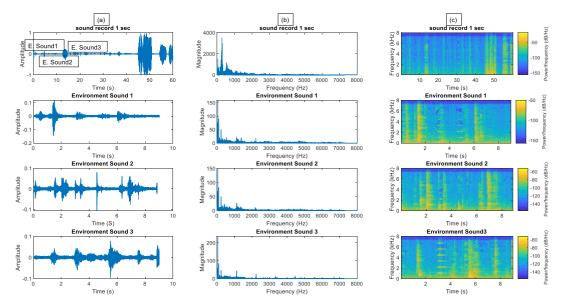
Figure 6. Environment sounds analysis represented in (a) time domain (b) frequency domain (c) spectrogram
