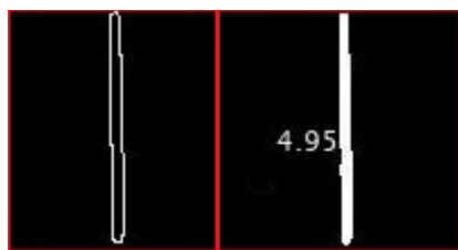
Fig. 8. Edge detection and gap width measurement output
