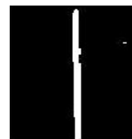
Fig. 7. Weld path image cleared of noise
